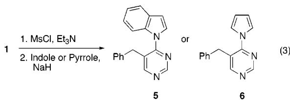
as the nucleophile under the same reaction conditions, the 4,5-disubstituted pyrimidine **5** was obtained in 61% yield after purification. We also examined the use of a less stable heterocycle, pyrrole, in this new method. We were gratified to find that the 4,5-disubstituted pyrrolypyrimidine **6** was obtained in 35% yield after purification. The NMR spectral assignments for **5** and **6** followed from those determined for compound **2**.
